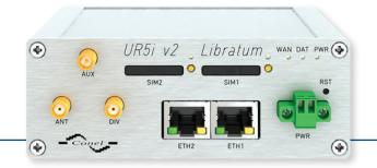
Balanced UR5iv2 Libratum a UMTS/HSPA+, non-modular wireless router features high speed data rates 14.4 Mbps, two Ethernet 10/100 ports and dual-SIM failover capability for mission critical applications. This router is particularly suited to the demands of the "Transaction Management" industry such as point-of-sale terminals, remote ATMs and vending terminals as well as a huge variety of intelligent remote monitoring and control applications in the Transport, Energy and Security sectors.
