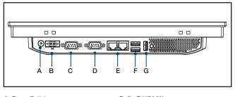
A. Power Switch B. DC-In C. RS-232
