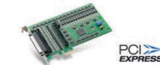
PCIE-1730 32-Channel TTL and 32-Channel Isolated DI/O PCI Express Card
